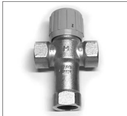
Figure 23 - Adjust Thermostatic Mixing Valves at each point-of-use to 120°F/49°C or lower.
