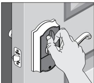
2. Rotate the thumbturn back to the horizontal position to re-lock.
